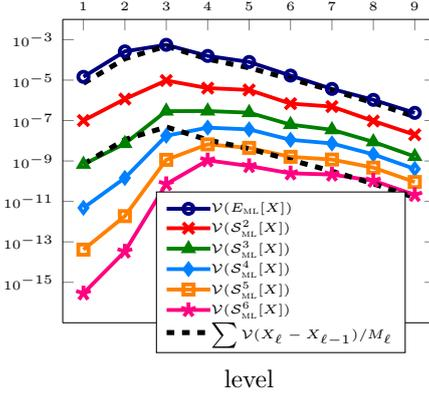
**Fig. 11** The variance of the Multilevel Monte Carlo estimators for the first six moments. The slope of the dashed lines represents the decay of the asymptotic upper bound.
