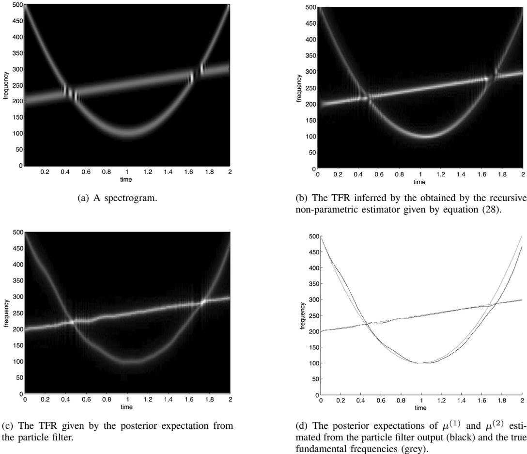
Fig. 1: Analysis of the first signal.
