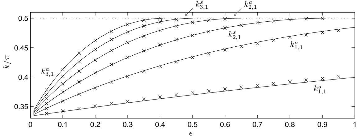
Figure 2: Trapped mode wavenumbers for the duct profile (3.6) with  $h_1 = 1.5$ , plotted as a function of  $\epsilon$ . Solid lines denote solutions of (3.4) and (3.5), as labelled; symbols denote solutions of the full problem determined via the spectral method.
