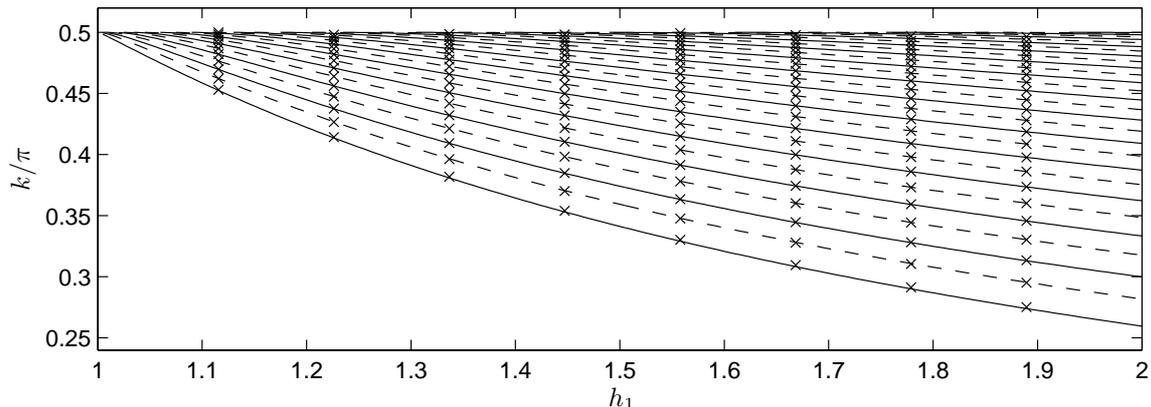
Figure 1: Wavenumbers for the symmetric (solid line) and antisymmetric (dashed line) trapped modes for the duct profile (3.6), plotted as a function of the bulge half-width  $h_1$ . Here,  $\epsilon = 0.1$ . Symbols denote solutions of the full problem determined via the spectral method.
