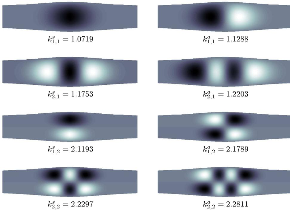
Figure 3: Structure of the first eight trapped modes, given from the uniform expansion (2.47), for the duct profile (3.6) with  $\epsilon = 0.1$  and  $h_1 = 1.5$ .
