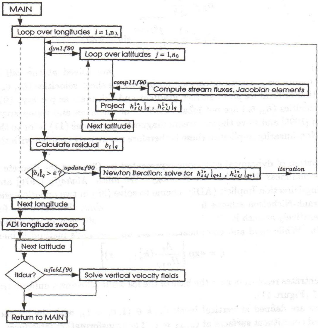
Figure 10. Flowchart of the dynamical system.
