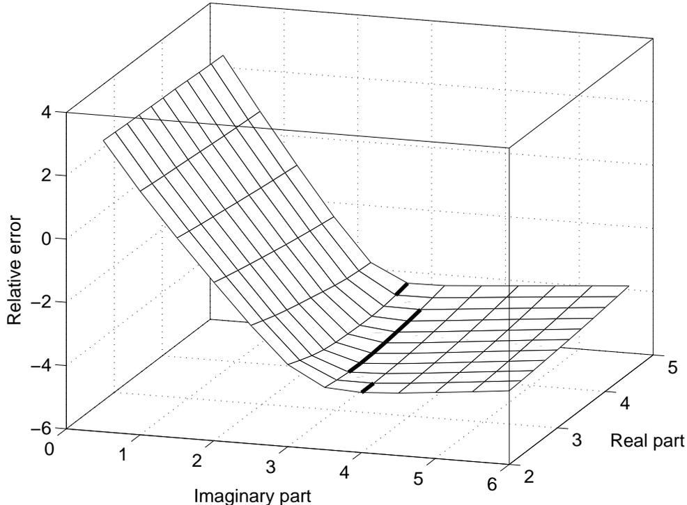
FIG. 6.2. A surface plot of the base 10 logarithm of the discrete relative  $L^2$  error for the PML/finite element solution against the real and imaginary parts of  $\tilde{L}$  (using a Neumann boundary condition on the PML). The solid line marks the minimum error for fixed real part as the imaginary part is varied. Clearly this graph suggests exponential convergence as the imaginary part of  $\sigma$  increases and almost no dependence on the real part.
