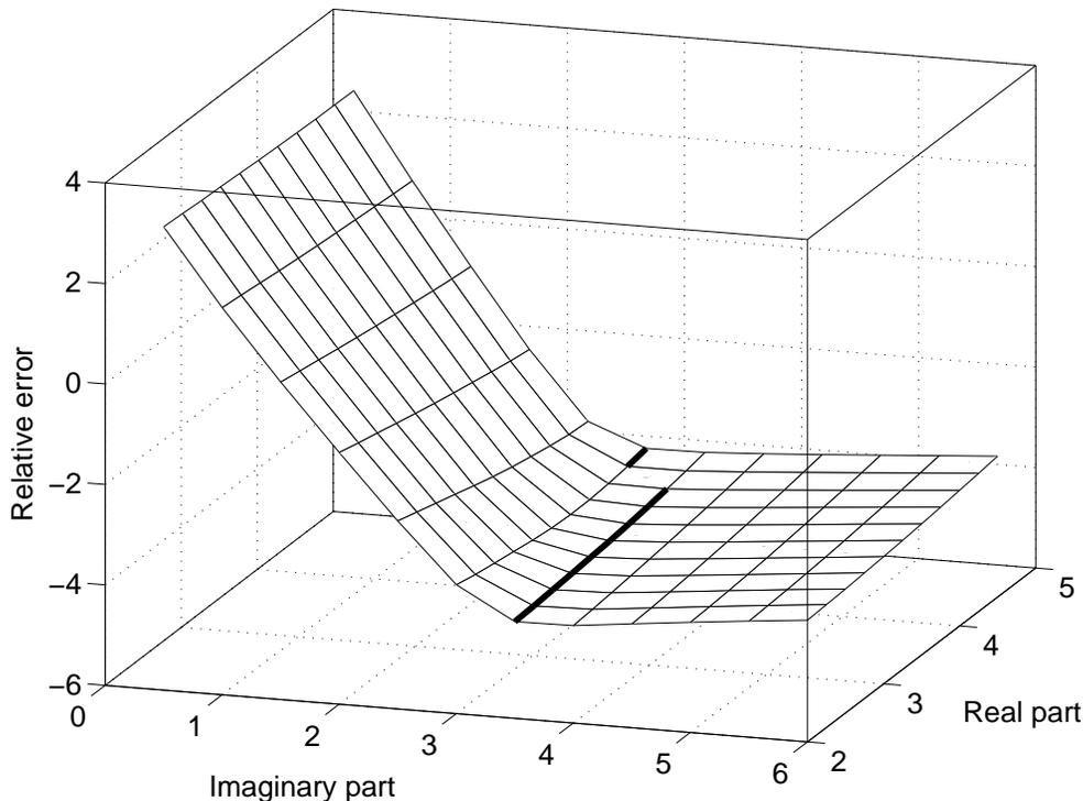
FIG. 6.3. A surface plot of the base 10 logarithm of the discrete relative  $L^2$  error for the PML/finite element solution against the real and imaginary parts of  $\tilde{L}$  using the homogeneous Dirichlet boundary condition on the PML. Generally the results are similar to those computed using the Neumann boundary condition in Fig. 6.2.
