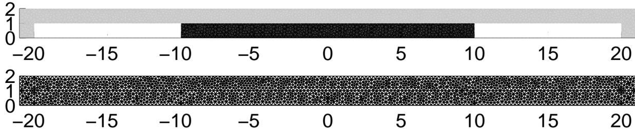
FIG. 6.1. The top panel shows the domain of the computation. The gray region is PML. The black and white regions are the truncated  $S_H$  and the black region is where the error between the exact and PML/FEM solution is computed. The lower figure shows the mesh which is very fine since we wish to study effects of the PML rather than the mesh.
