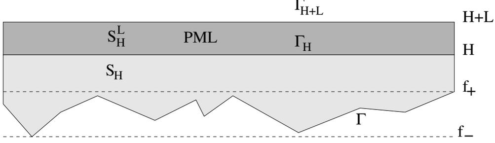
FIG. 2.1. A schematic showing some of the notation for the PML terminated acoustic rough surface problem. The lightly shaded region  $S_H$  is the main computational domain where the Helmholtz equation is satisfied. The domain  $S_H^L$  is occupied by the PML. A non-homogeneous Dirichlet boundary condition is applied on  $\Gamma$  and a homogeneous Neumann condition is applied on  $\Gamma_{H+L}$ . The boundary  $\Gamma_H$  is used in computing the Dirichlet to Neumann maps.
