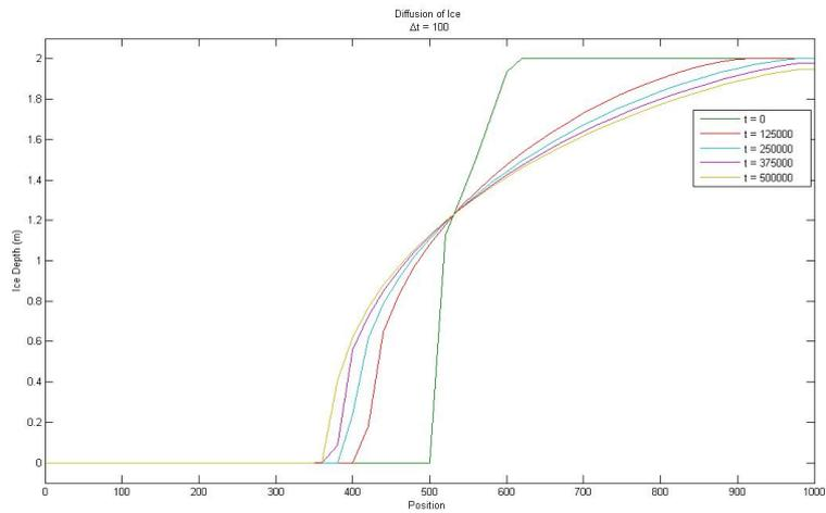
Figure 4.4: Diffusion in a 2m slab of pack ice with a parabolic front
