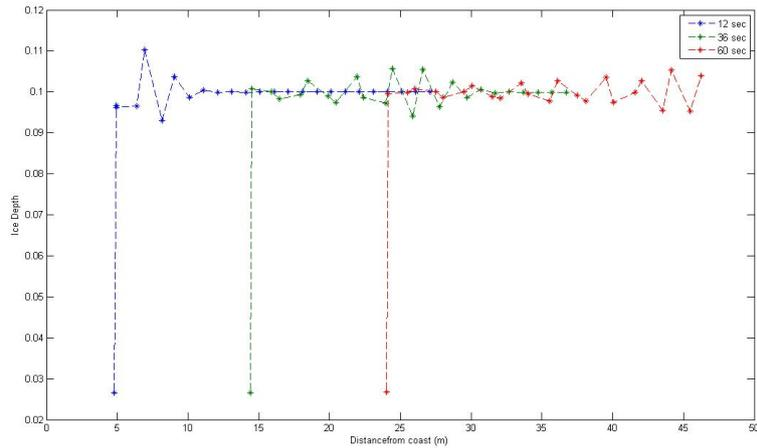
Figure 5.4: Initial sixty seconds of the moving grid model, illustrating the instability.
