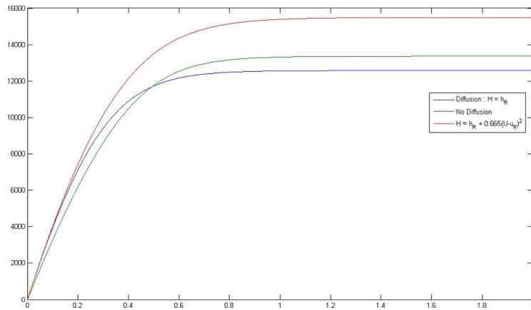
Figure 5.5: Comparative opening phase for a polynya with and without the altered boundary condition, wind speed is  $20\text{ms}^{-1}$
