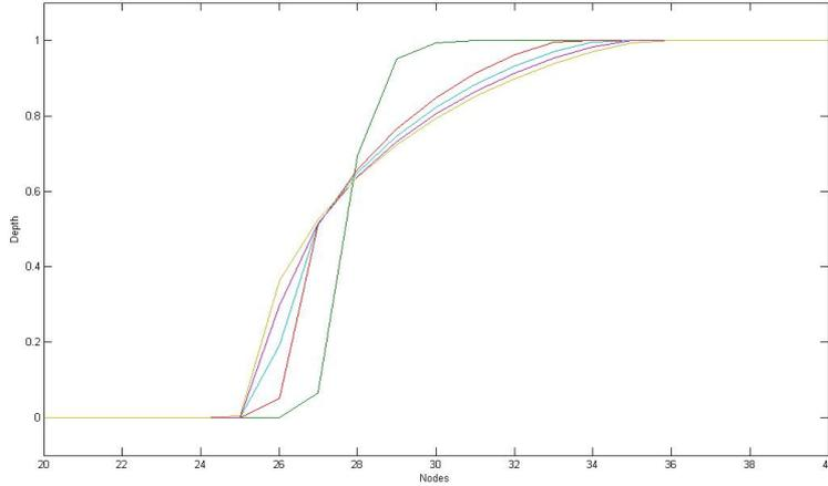
Figure 4.5: Diffusion in a 1m slab of ice which has a  $\tanh$  curve defining the shape of the ice for its initial conditions
