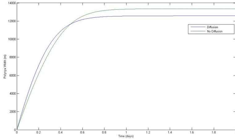
Figure 4.7: Comparative opening phase for a polynya with and without the ice diffusion included in the parameterisation, wind speed is  $20ms^{-1}$
