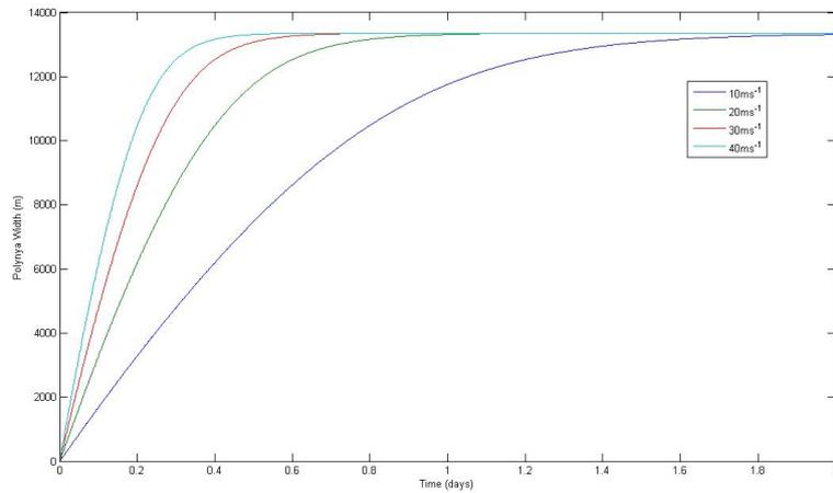
Figure 3.3: Runge-Kutta fourth order, showing the effect that varying the wind speed has on the polynya when temperature is kept constant at  $-20^{\circ}C$
