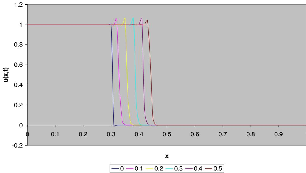
Figure 5-5: Lax-Wendroff approach applied to (5.1) with  $\mu = 1000$ .
