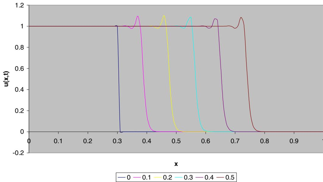
Figure 5-4: Lax-Wendroff approach applied to (5.1) with  $\mu = 100$ .
