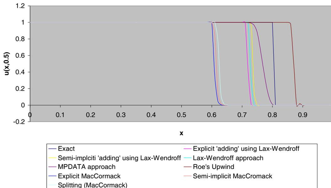
Figure 5-20: Comparison of second order schemes with TVD listed in Table 5-1 with stiff source term.
