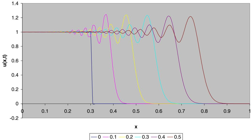
Figure 5-2: Lax-Wendroff approach applied to (5.1) with  $\mu = 1$ .
