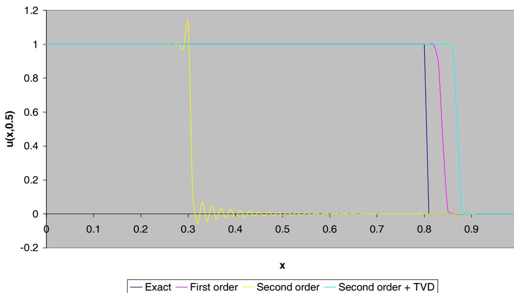
Figure 5-12: Roe's Upwind approach with stiff source term.
