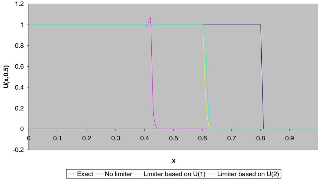
Figure 5-15: Semi-implicit MacCormack approach with stiff source term.
