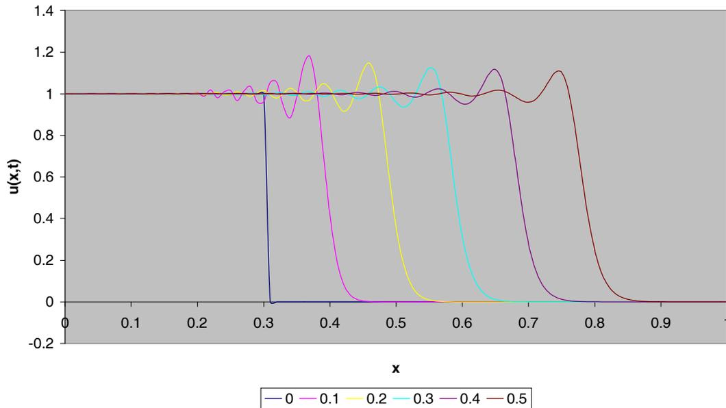
Figure 5-3: Lax-Wendroff approach applied to (5.1) with  $\mu = 10$ .
