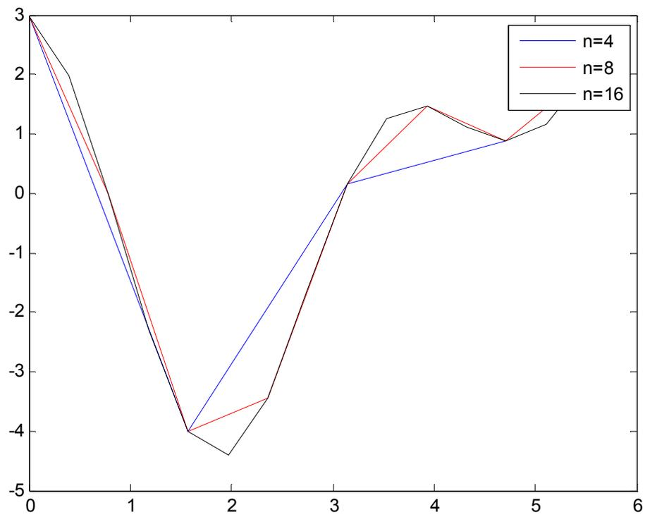
Figure 6.1: The numerical solution of the full pipe flow problem for  $n=4,8,16$ .
