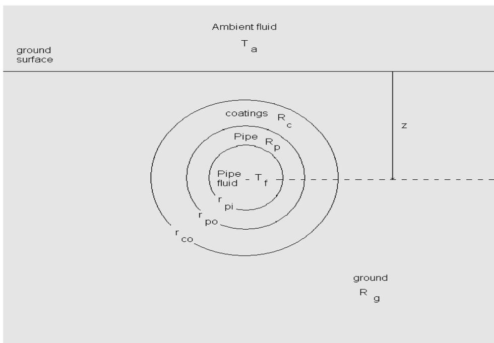
Figure1: Buried pipe (source: Partially Buried Pipe Heat Transfer (Powerpoint), Chuk Ovuworie from Schlumberger Company)
