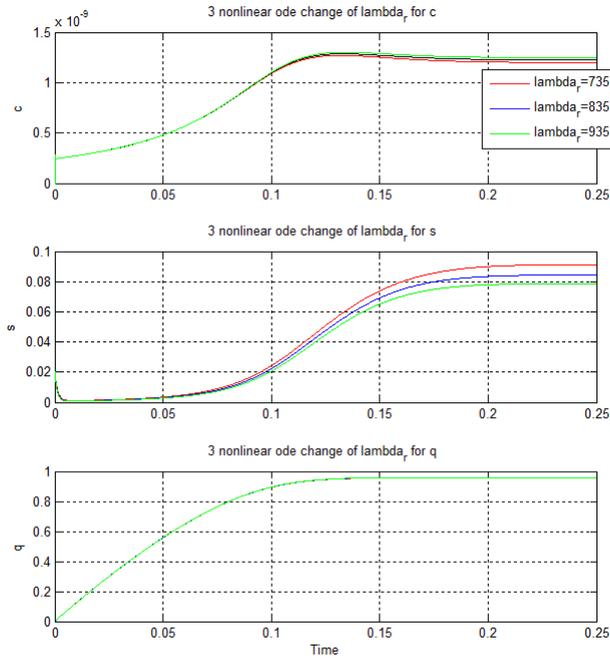
Figure 7.3: Change of  $\lambda_r$  for  $c$ ,  $s$  and  $q$  in 3 ODEs.
