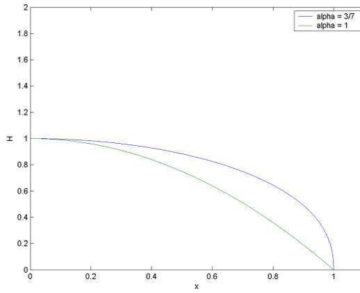
(c) Initial Ice Thickness under different  $\alpha$
