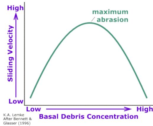
**Figure 8.1:** *Effect of Abrasion on Basal Sliding*
